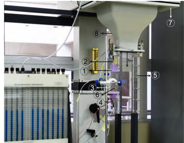
Figure 5. Test section assembly attached to flow bench (flow direction is vertically downwards). Numbered components show the (1) front wall, (2) front wall microphone, (3) cavity, (4) aft wall microphone, (5) rectangular test section with embedded cavity, (6) piezoelectric beam, (7) settling chamber and (8) converging nozzle.
