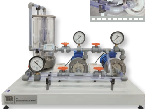
SERIES AND PARALLEL PUMPS (H52)
