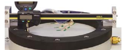
DEFLEX®-3D VISUALISATION OF THE EFFECT OF PRESSURE ON THE SURFACE PROFILE OF THE SM1008 DIAPHRAGM
